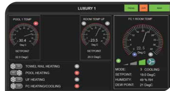
Data screen for Luxury Villa 1 on PLC control system.
